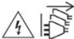
The system may have one or more power supply unit (PSU) cords. To avoid serious injuries, it is recommended that all PSU power cords must be disconnected by trained service technicians before installing or replacing system components.
