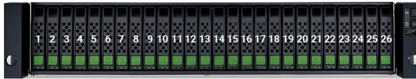
Figure 2-2 Disk Drive Numbering
