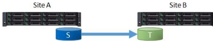
Figure 4-12 One-Directional Remote Replication
