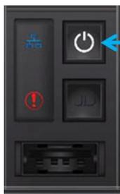
Press and hold the power button for **4 seconds** to power off the system
