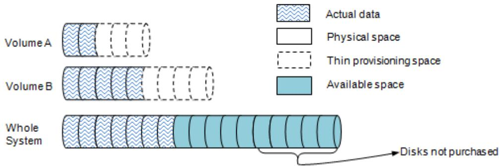
Figure 9-2 Thin Provisioning
