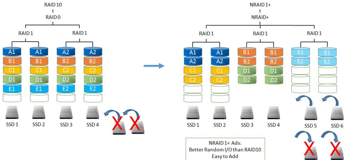
Figure 10-5 SSD Read-write Cache with NRAID 1+
