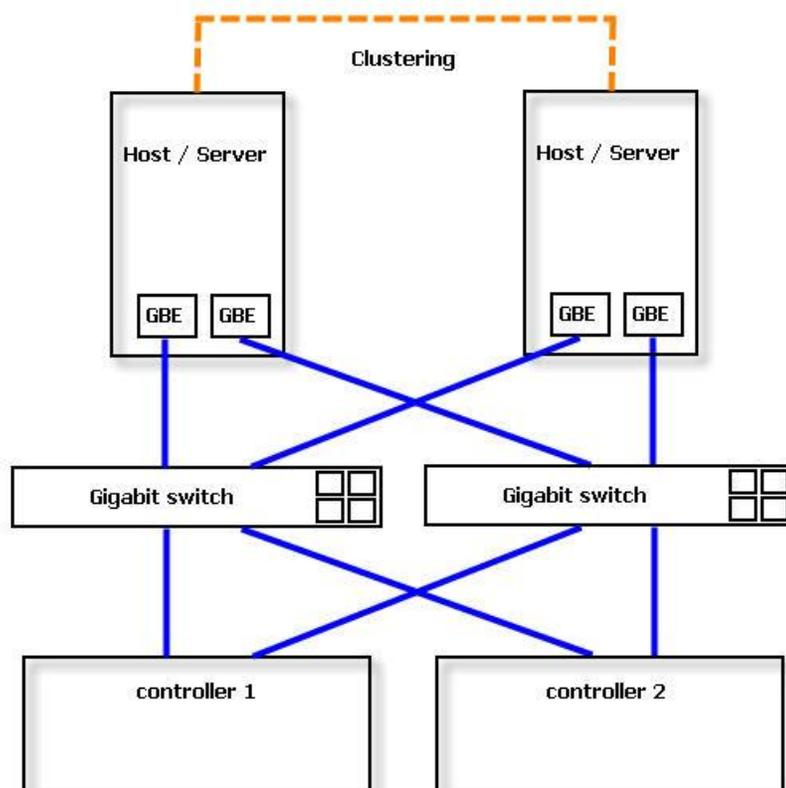
Figure 2-1 Dual-controller Topology
