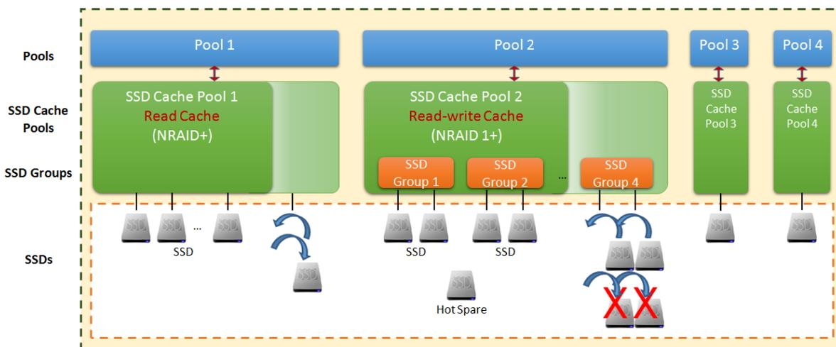
Figure 10-2 Storage Architecture of SSD Cache Pool
