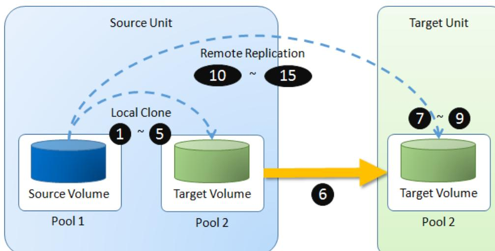
Figure 12-51 Local Clone Transfers to Remote Replication Diagram
