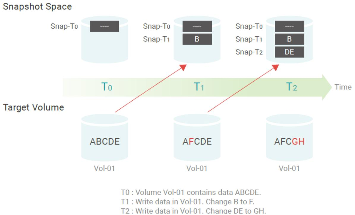
Figure 12-1 Copy-on-Write Technology
