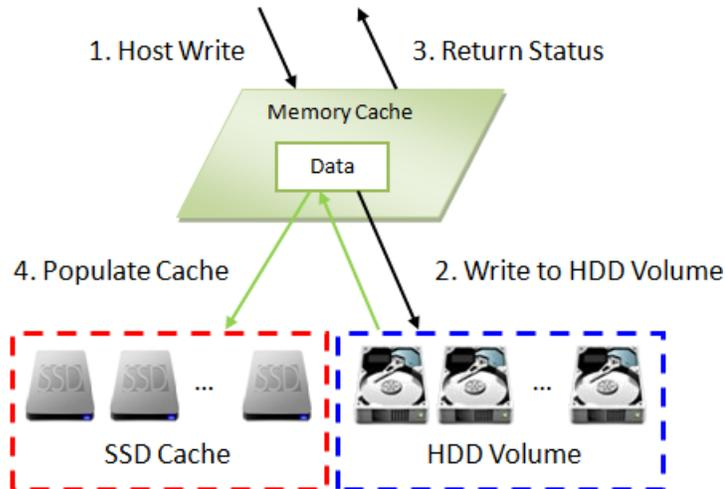
Figure 10-8 Write Data in SSD Read Cache
