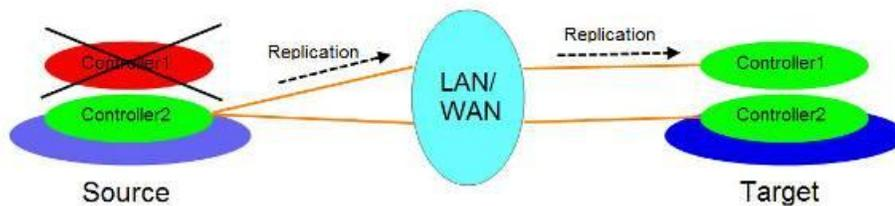
Figure 12-42 Remote Replication Source Controller Fail Diagram
