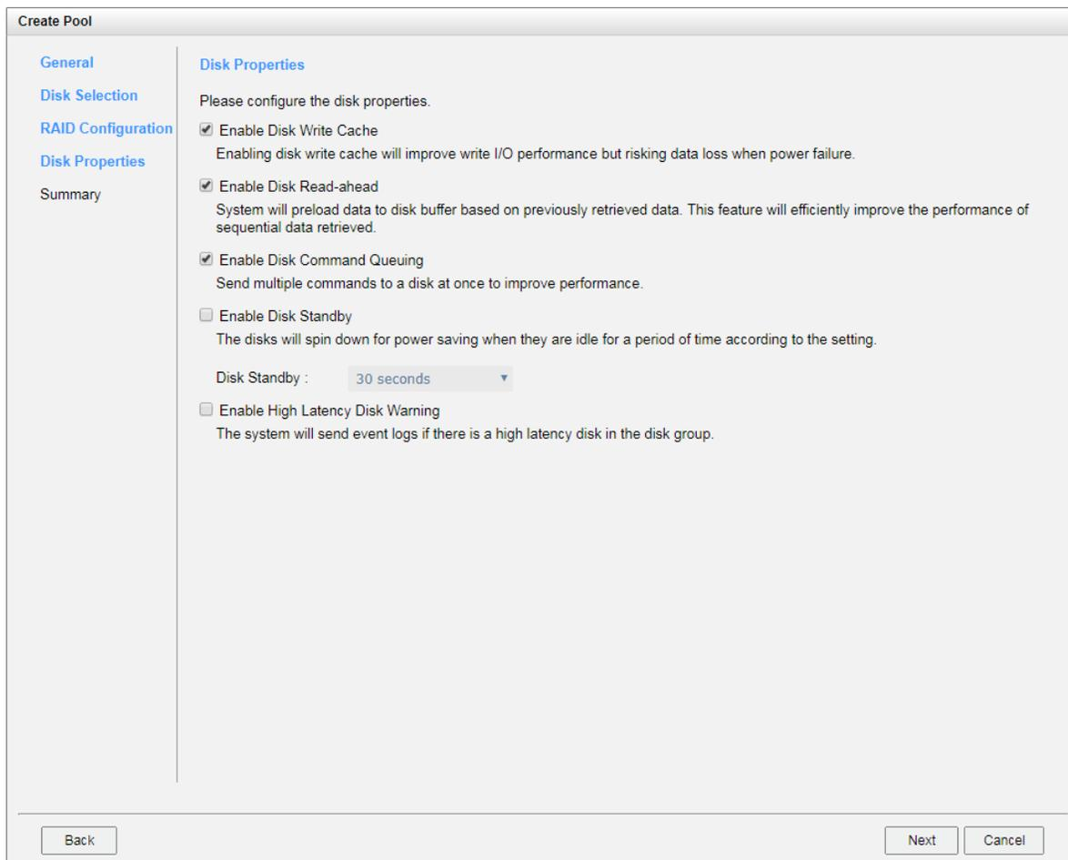
Figure 8-23 Create a Thick Provision Pool Step 4
