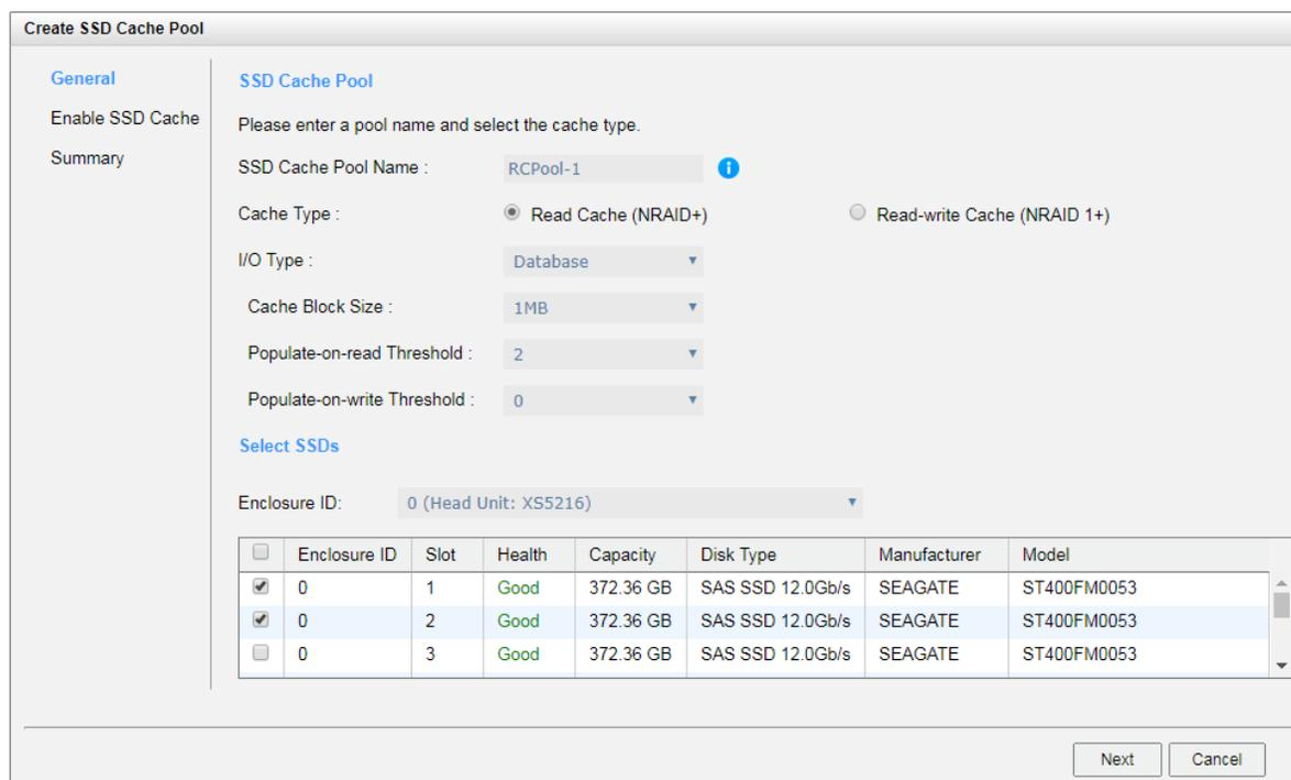
Figure 10-12 Create an SSD Cache Pool Step 1
