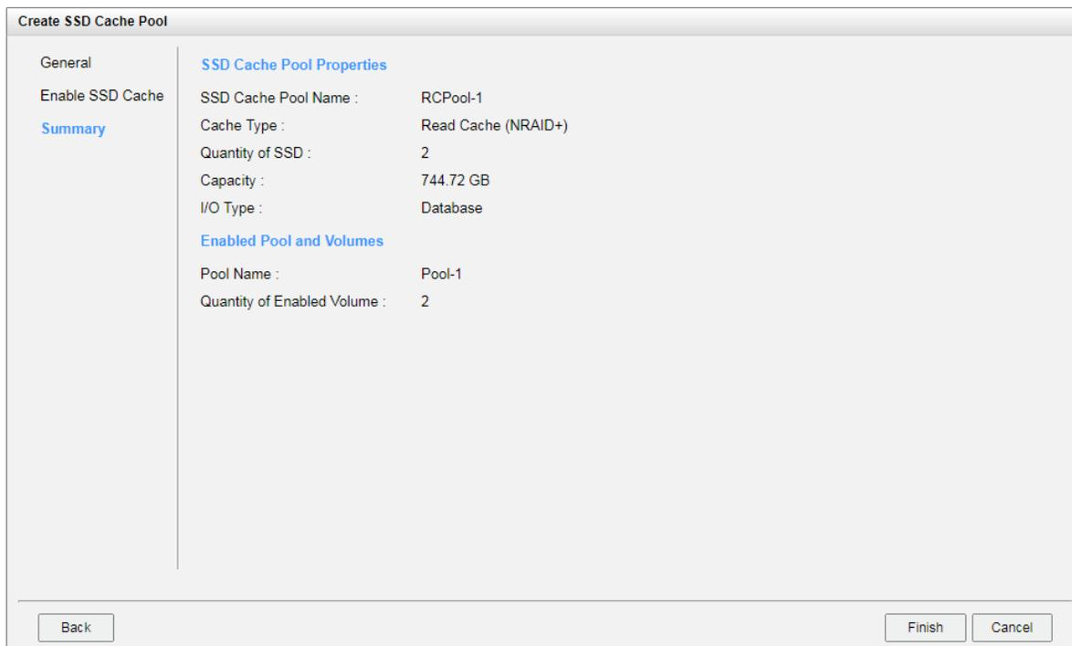
Figure 10-14 Create an SSD Cache Pool Step 3
