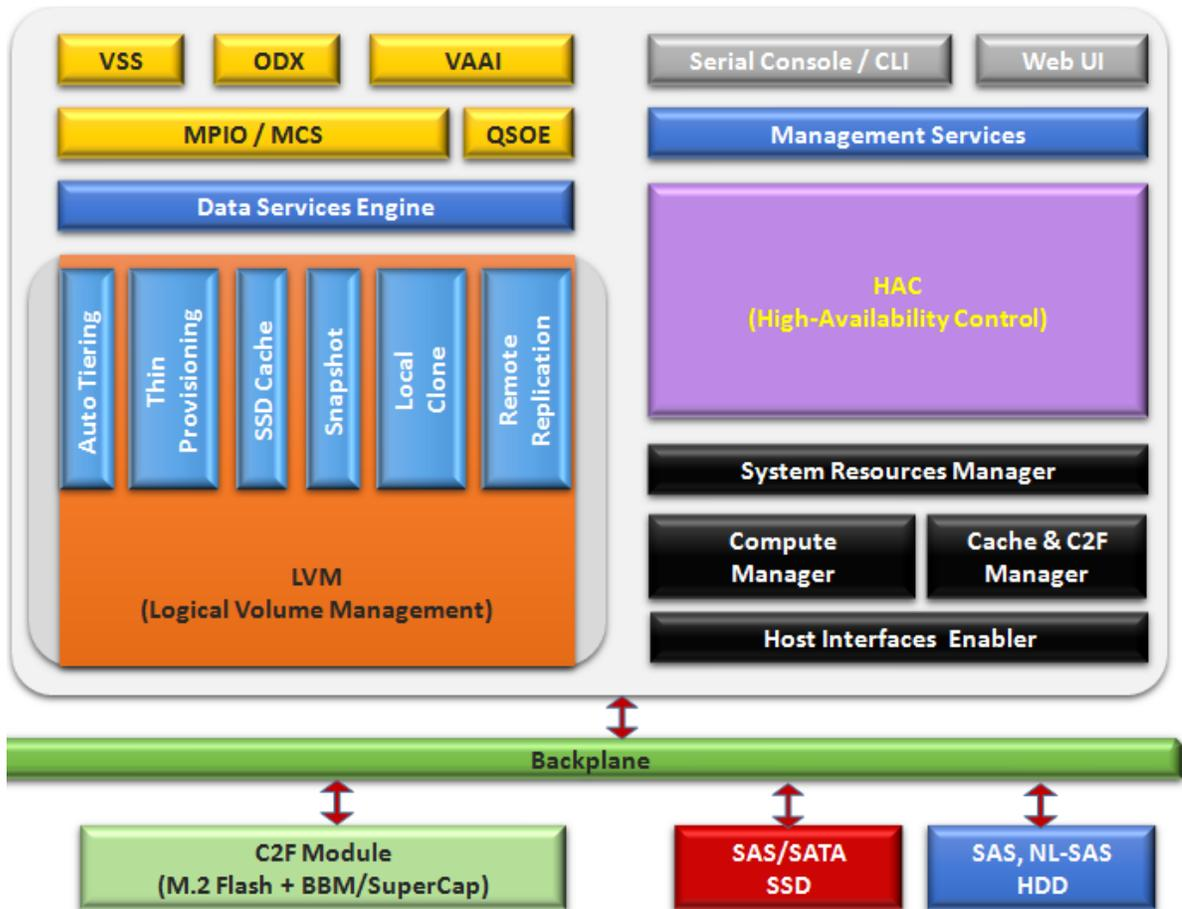
Figure 1-2 SANOS System Architecture with Single Controller Configuration
