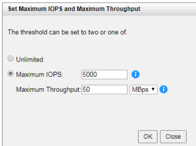
Figure 15-11 Set Maximum IOPS and Maximum Throughput
