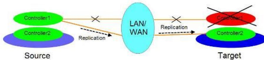
Figure 12-43 Remote Replication Target Controller Fail Diagram
