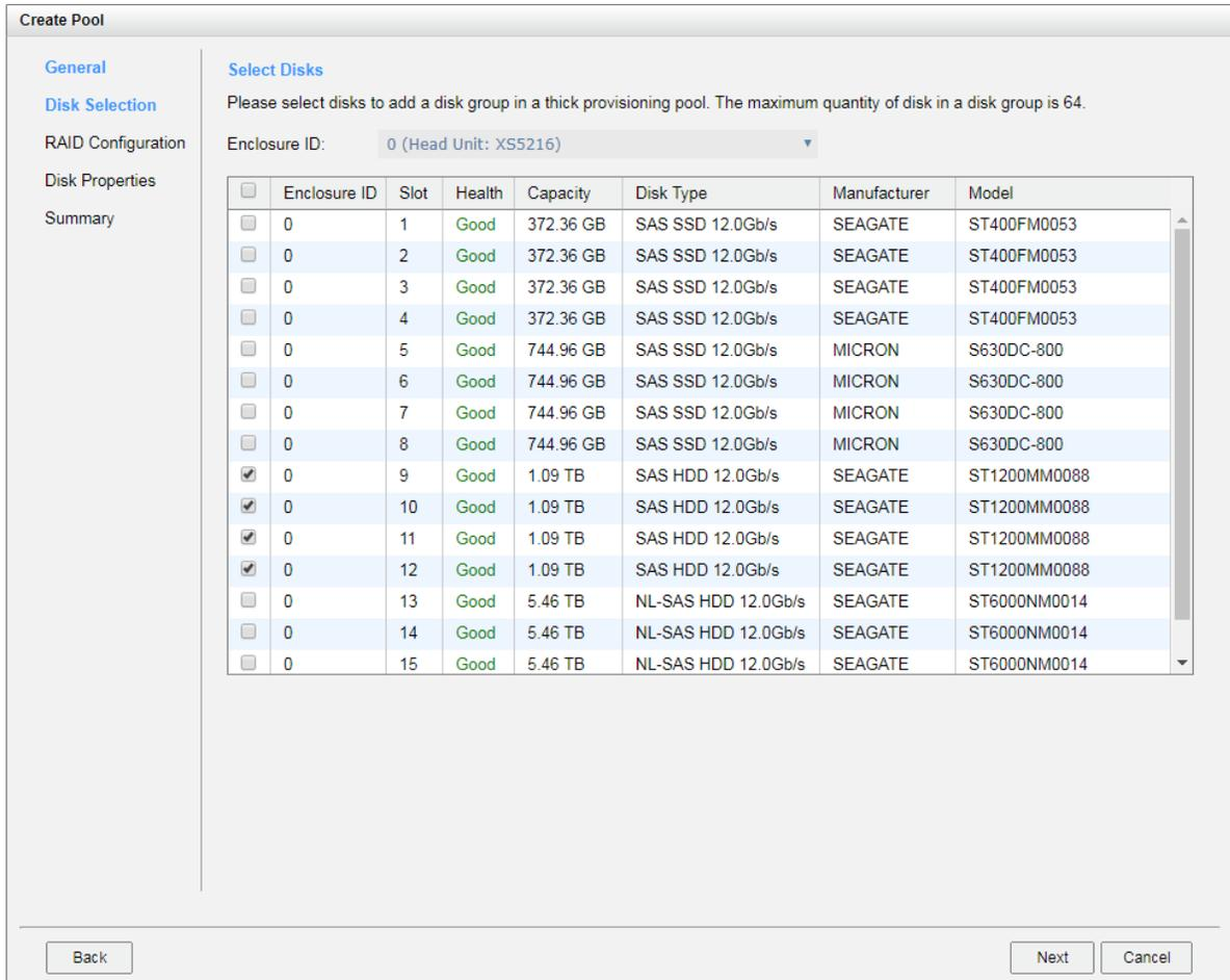
Figure 8-21 Create a Thick Provision Pool Step 2
