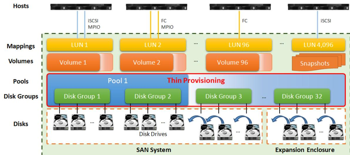
Figure 9-4 Storage Architecture of Thin Provisioning Pool
