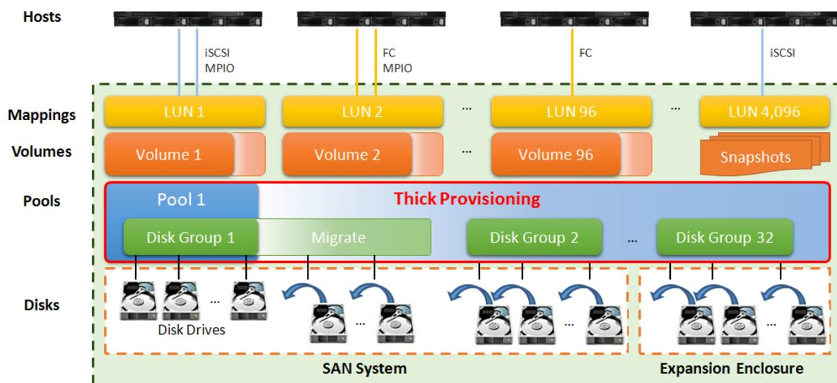
Figure 8-6 Storage Architecture of Thick Provisioning Pool
