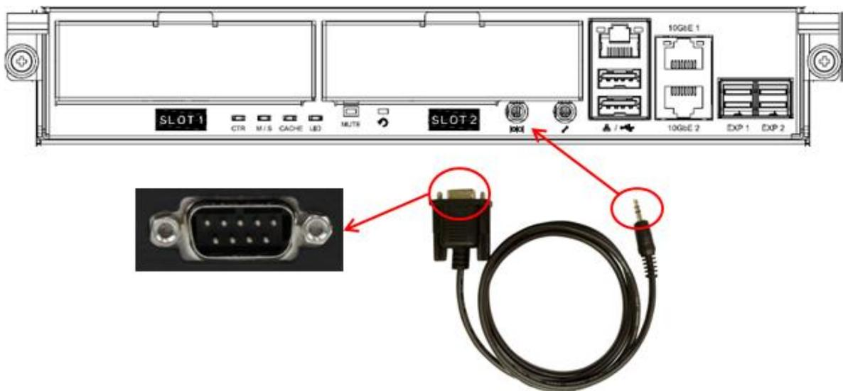
Figure 17-3 Connect the Console Cable
