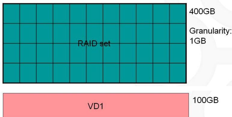
The RAID set will be divided by the Granularity (1 GB) which is the minimum size while allocating the space to a VD.
