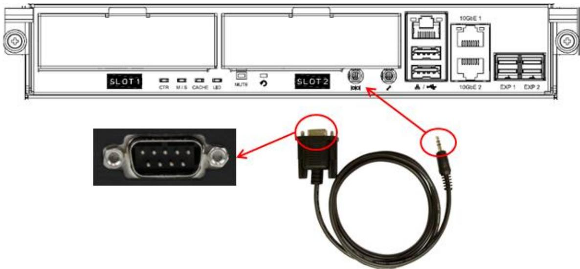
Figure 11-3 Connect the Console Cable
